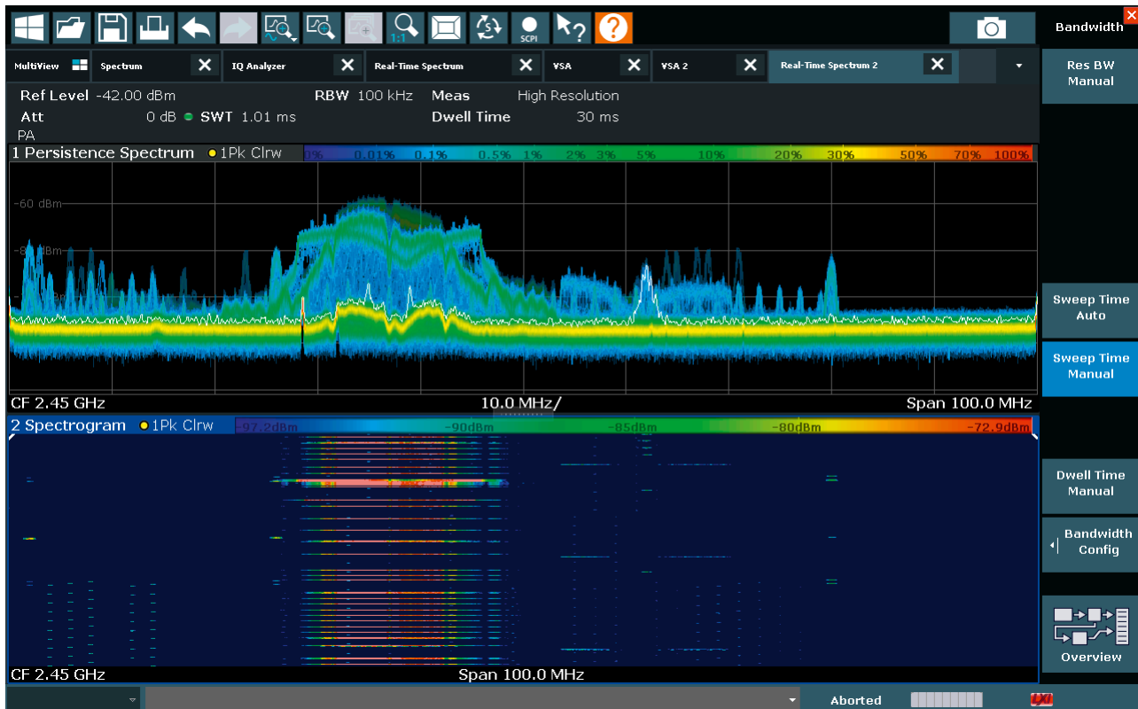
Real-time spectrum of the ISM band at 2.4 GHz
